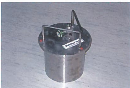
Shielding and stainless steel container for ^{226}\text{Ra} samples: blue Pb shielding with inner and outer containers (top left), container set (top right), Pb shielding in inner container (middle left), sealed inner container in outer container (middle right), complete set of shielding with inner and outer container (bottom left).
